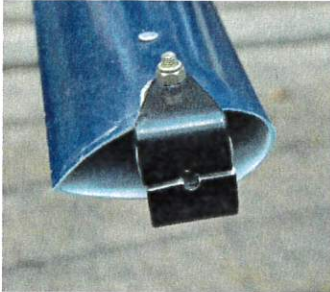
Figure 1. Fractured right front lift strut bracket
