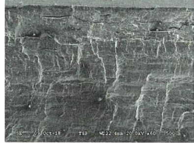
Figure 3. Secondary and parallel cracks underneath the surface of the bracket
